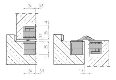
Section of Wood Frame-Door Installation
