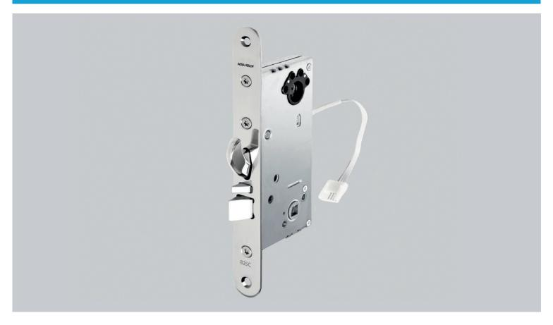
The ASSA ABLOY handle controlled motor locks are part of a family of multi-functional motor locks with two main types and five variants: The 825C-50 features an electronically controlled deadlatch (adjustable split spindle) and a mechanical hook bolt that provides increased holding force with auto retract function, it is certified according to EN179 which allows installation in escape routes.
