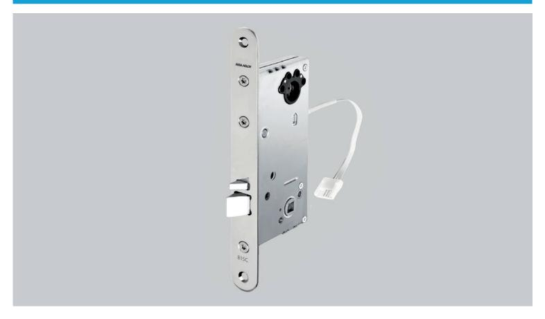
The ASSA ABLOY handle controlled motor locks are part of a family of multi-functional motor locks with two main types and five variants: The 815C-50 features an electronically controlled deadlatch with an adjustable split spindle for electronic entry and mechanical exit, it is certified according to EN179 which allows installation in escape routes.
