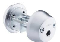
**Product description**Single inside cylinder to be used with mortice lock cases for standard doors, both mechanical and electric lock cases.
